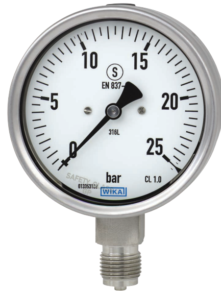
Bourdon tube pressure gauge, model 232.30, NS 100 [4"]
