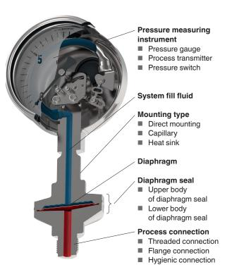
Installation example of a diaphragm seal system
