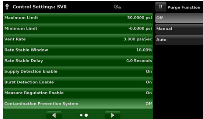
Fig. 8.9.2.3-B - Contamination prevention system
