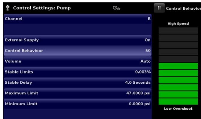
Fig. 6.4.3.3 - Control behaviour for pump module
